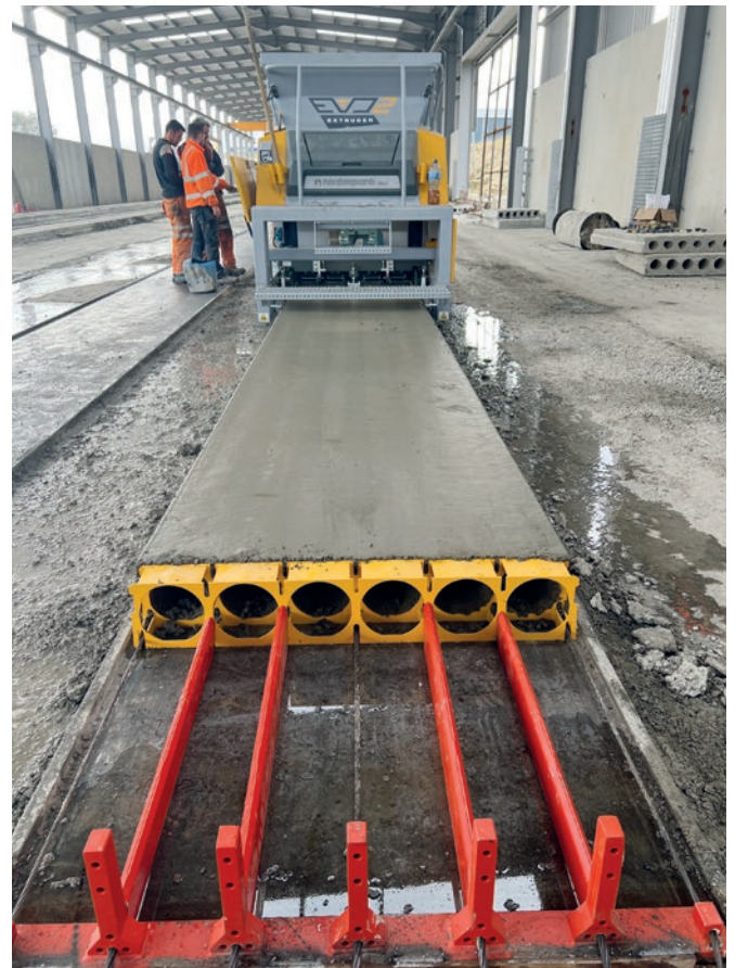
EVO2 extruder during the casting phase
